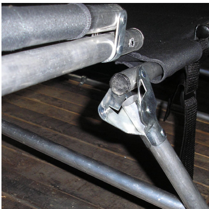
Failure at 2780 cycles
